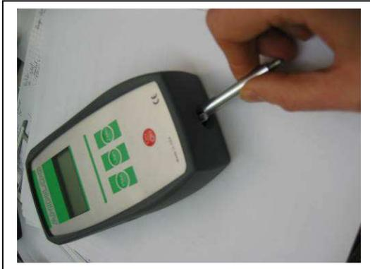
Affix the extension rod to the load cell probe in the hole at the bottom of the gauge by tightening it gently with the fingers.
