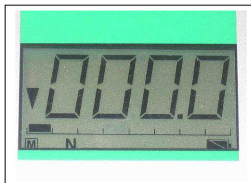
If a force of more than 20% of the maximum capacity is applied via the load cell probe (hole at bottom of CENTOR FIRST), the display will show 'OVERLOAD'
