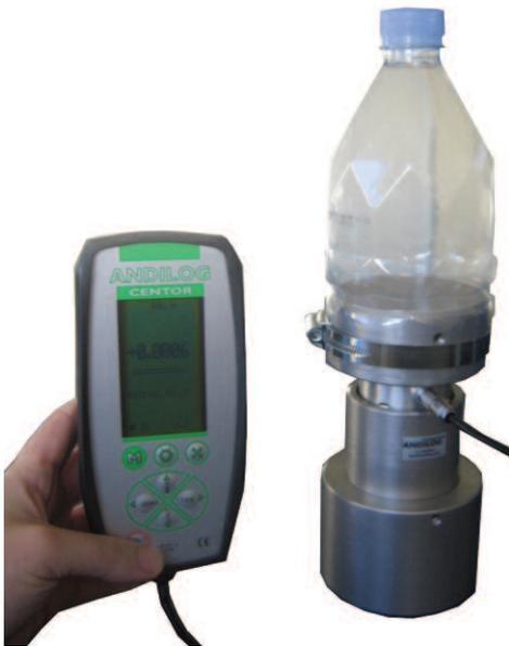
Instrumented bottle to measure the capping torque. The mechanical support includes the torque sensor and has been designed according to the bottle shape
