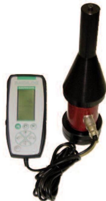
Instrumented bottle to measure the insertion force for champagne capping machine with a force sensor up to 10kN
