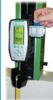
Datastick compatible : Memory card reader to save your data (curve, peak, calculation) to a SD memory card. The test stand doesn't have to be connected to a computer while you do your tests.
