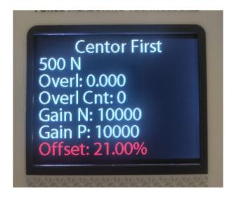
All settings are saved in memory when the force gauge is turned off. The force gauge will operate with the same settings when it is turned back on (unit, display order).
