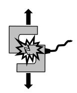
It is important that the measured values are generally below 90% of the sensor's capacity. Constant use of the load cell beyond 90% of its capacity can result in premature wear of the load cell. When the force gauge is used on a motorized frame, it is necessary to program the frame to stop when the force approaches the maximum capacity of the sensor. This limit must take into account the fact that at a
