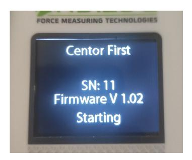
After the self-test, if the device is functional, the force gauge displays the measurement screen. It then displays 0 N. A tare is performed when the device is started.
